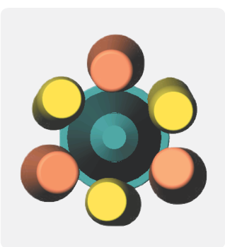
Optimal roll alignment for fast rolling. Maximum roll to tube contact reducing spring back effect. Equal load distribution leading to extended expander life.
